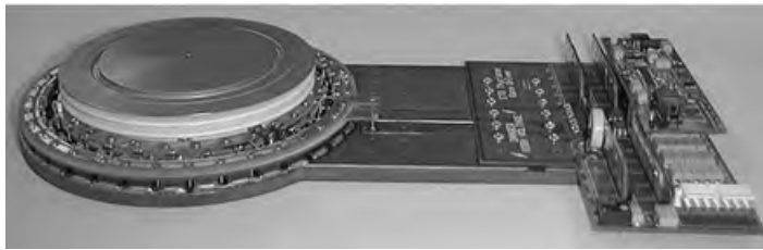
FIGURE 1.99 ETO equivalent circuit (a) and a 4-kA/6-kV ETO (b). An ETO gate driver is also shown.
